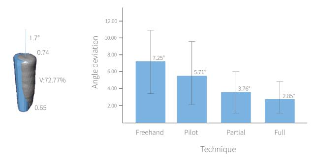
The results regarding angular deviation are summarized in the figure above (values are shown as mean angular deviation  $\pm$  SD).
